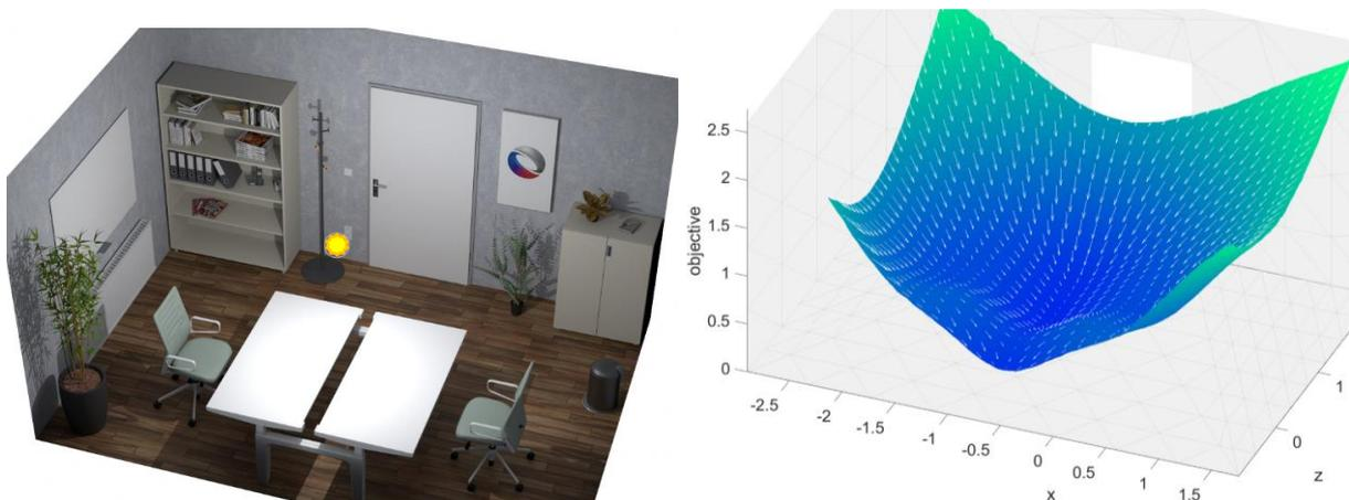
Example: positioning a light source such as to illuminate two desks in a small office; right: the cost function to be optimized and its gradient. With more complex scene layouts, local minima become increasingly problematic, requiring more robust and efficient design methodology.
