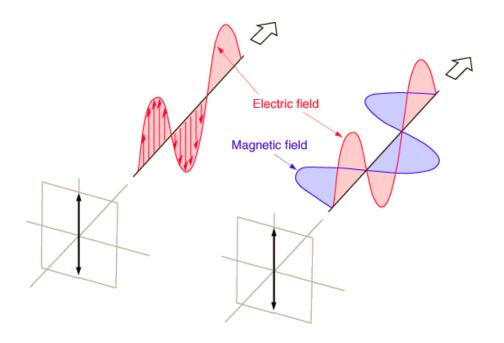
Circularly polarized light consists of two perpendicular electromagnetic plane waves of equal amplitude and 90° difference in phase.
