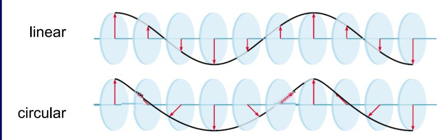
Circular polarized light oscillates only in one rotating direction
