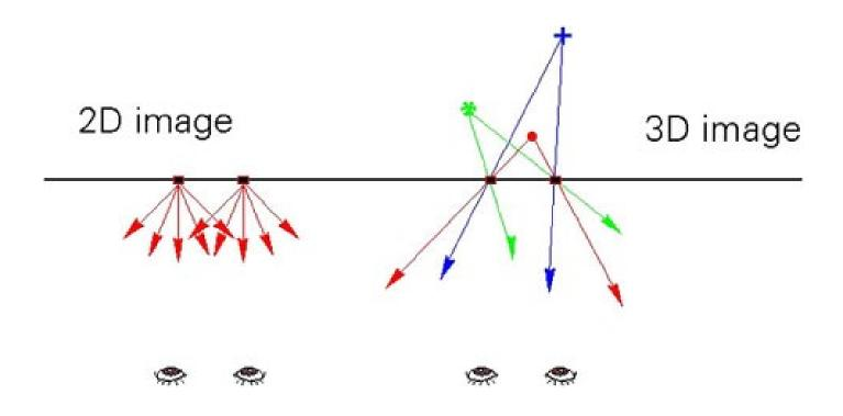
pixels on screen send different light in different direction, thereby simulating light emanating from points in space:
