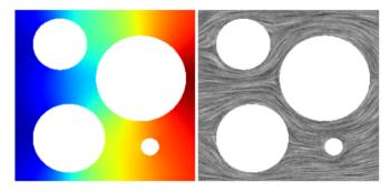
Fig. 9. Potential flow reconstruction from the velocity boundary condition.
