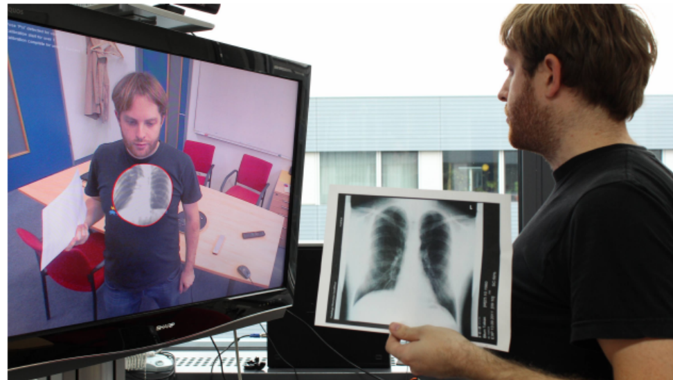
Figure 1: An X-ray is augmented onto the user. The X-ray is simulated from a CT of the same person. The printed image is a real X-ray of the same person.
