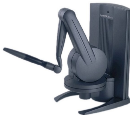
phantom tracking & haptic feedback device
