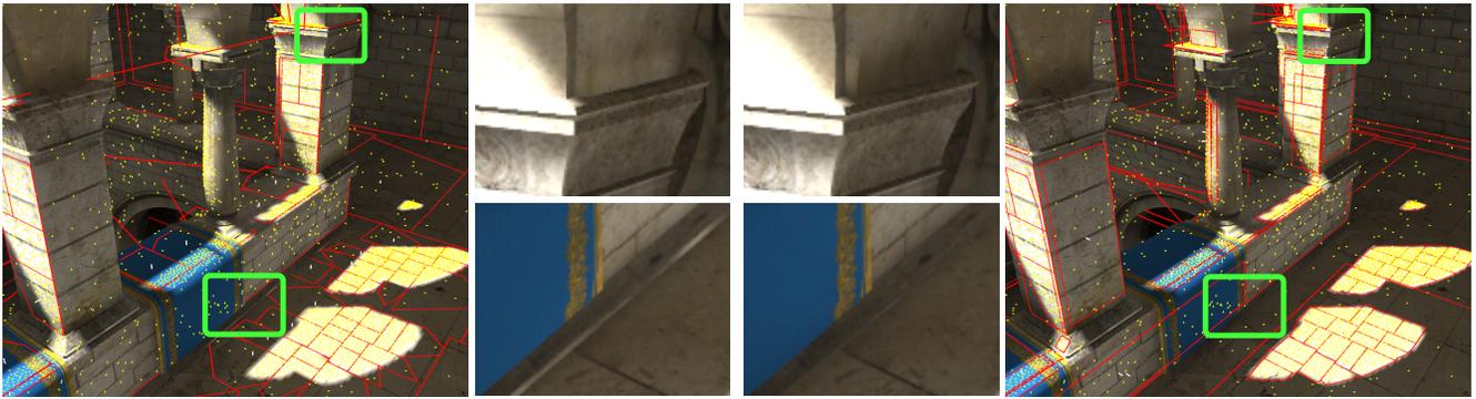
**Figure 9:** The left images are generated from clustering all bounces together, for the right images each bounce is clustered separately. Note the difference in the virtual light sources for the lit areas created by the direct illumination through the arches, and the incorrect illumination in the left two close-ups.
