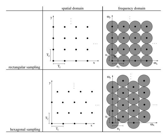
Figure 2: 2D regular rectangular and hexagonal sampling in the spatial and frequency domains.
