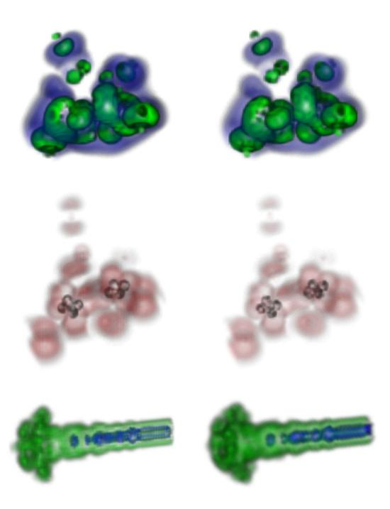
Color Plate 1: Images generated via splatting on a Cartesian grid on the left respectively a body-centered cubic grid on the right. The body-centered cubic grids require approximately 30% less samples. Small differences are visible, that likely are caused by pre-classification.
