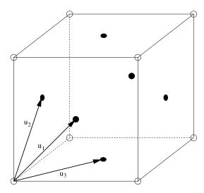
Figure 3: One cell of an fcc lattice with base vectors  $u_i$ . The black dots mark additional sample points (in the center of the faces) as compared to a simple cubic cell.
