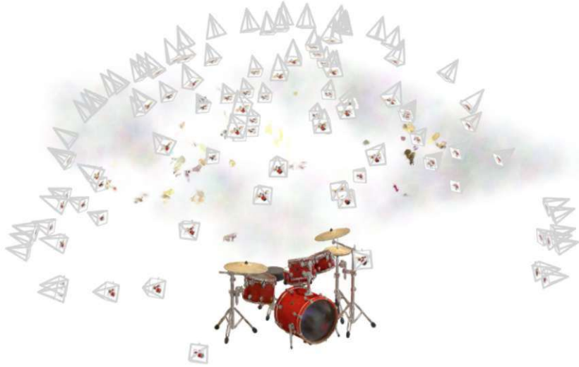
Figure 2.8: 3DGS reconstruction of the Drum scene from the NeRF Synthetic dataset, supervision images, and camera poses overlaid. Screenshot taken from NerfBaselines 3 .
