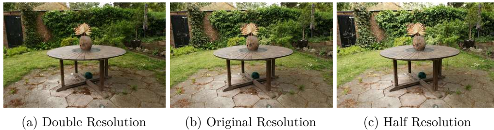
Figure 2.10: A 3DGS reconstruction at different resolutions showing aliasing. The same model of the Garden scene [13] was used to reconstruct the three images. The density of the Gaussians in the left image (a) rendered at twice the original resolution is too low, resulting in an overly dark appearance. The opposite effect is visible in the right image (c) rendered at half resolution, where the Gaussians are too wide, and the image appears too bright.
