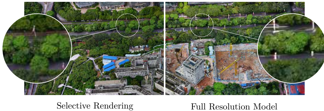
Figure 1.1: Demonstration of the method presented. A far view rendering of the ArtSci scene. Right: Image rendered with 3DGS uses 7.5 million primitives and exhibits aliasing. Thin structures appear too thick, and the overall appearance is too bright. Left: The selective rendering as presented in this thesis uses only 5.5 million primitives. Aliasing effects are reduced.
