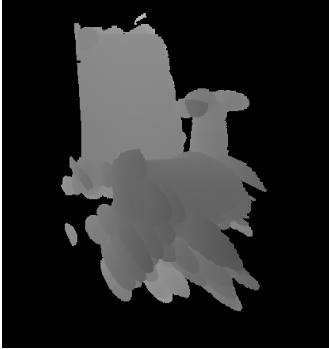
Figure 4.10: 3D Visualization of voxel towers after change detection, showing the Added intervals representing the changes between the two scenes.
