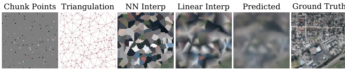
Figure 5.4: Example patch with inputs, processing steps, and network prediction.
