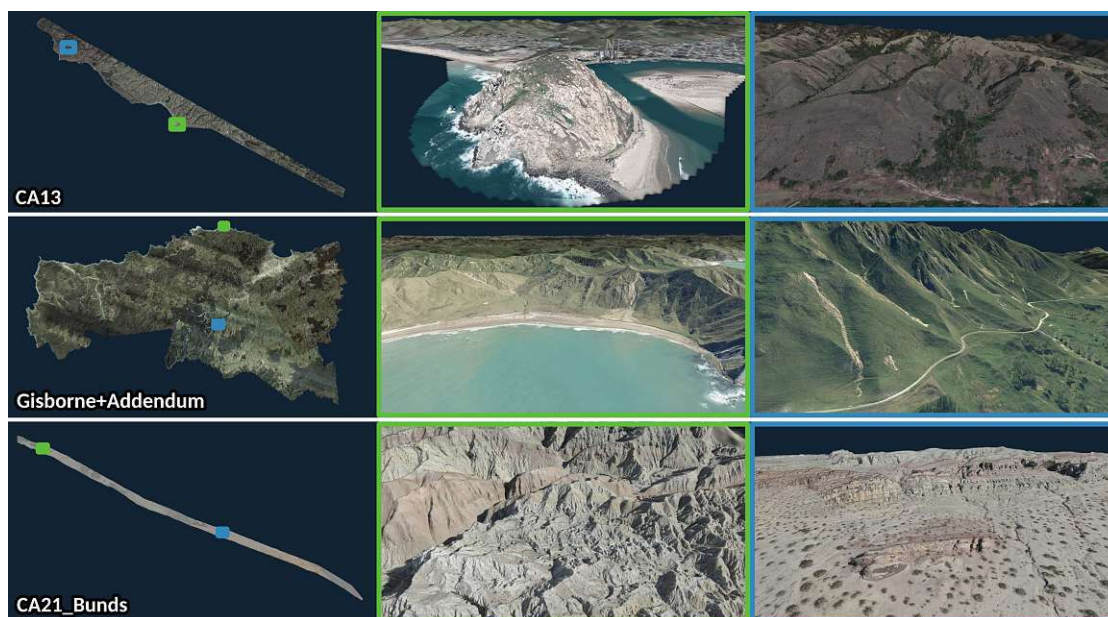
Figure 5.5: Screenshots of CA13 (17.7B points, 90GB), Gisborne (262B points, 2.4TB) and CA21_Bunds (8.4B points, 96GB) made with LIDARSCOUT.
