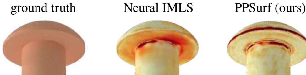
Figure 4.10: Limitations. Our method has difficulties to recover the edges of clean point clouds due to training with noisy point clouds.
