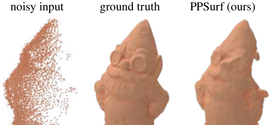
Figure 4.11: Limitations. Our method struggles with reconstructions of large missing areas in the input point cloud since we did not incorporate any generative model capabilities.
