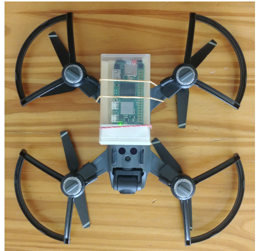
(d) Raspberry Pi Zero mounted along the length of the drone. Blocked sensors
