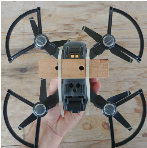
(c) Wood block with dimensions of Raspberry Pi mounted on its long side. Blocked sensors
