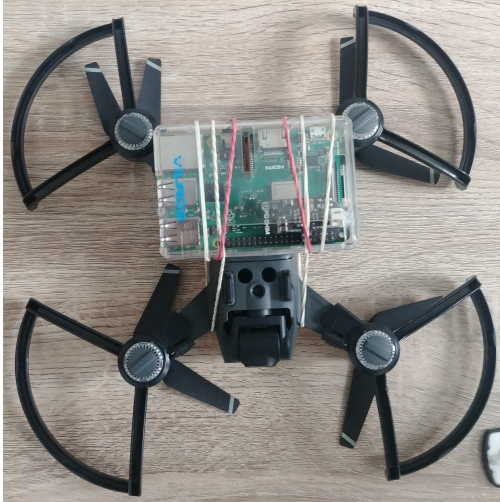
(a) Raspberry Pi centered. Blocked sensors
