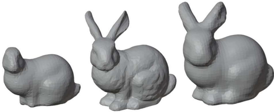
Figure 1.1: Shown here are the results from the algorithm with a constant offset, from left to right: the inner offset surface, the input surface and the outer offset surface. Both inner and outer offset surfaces were put through the DC rasterization phase and smoothed. A constant offset was used for both inner and outer offset surfaces. The octree generates leaves on the fifth level. The offset distance used for the output surface is 0.005.
