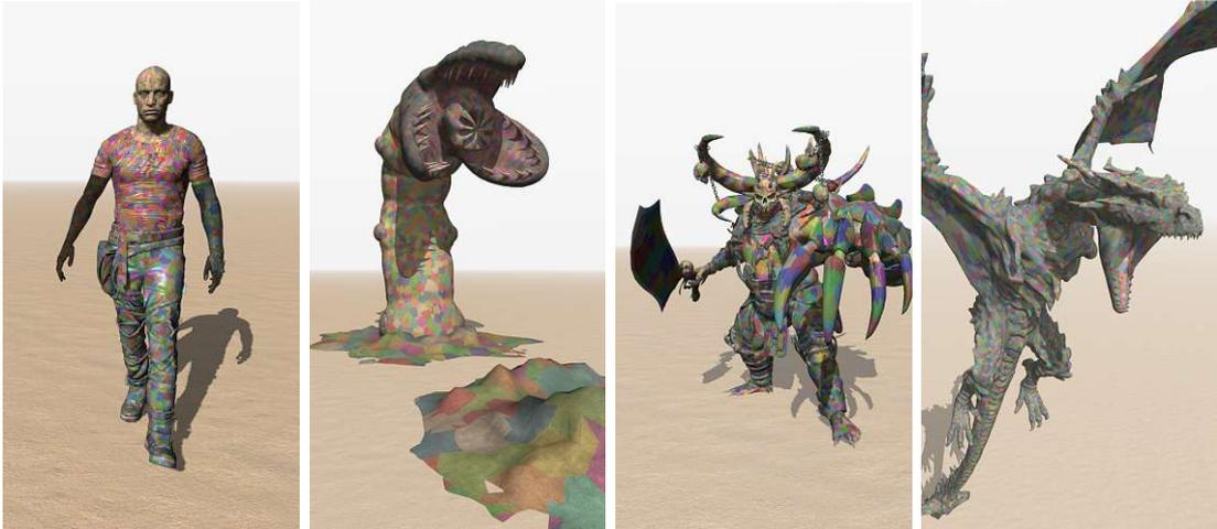
**Figure 4.1:** Skinned models GAWAIN<sup>1</sup> (198k vertices, 261k triangles, 136 bones, 9044 meshlets), GIANT WORM (169k vertices, 329k triangles, 80 bones, 10382 meshlets), BUTCHER (287k vertices, 477k triangles, 224 bones, 14915 meshlets), and WYVERN (267k vertices, 512k triangles, 88 bones, 16015 meshlets), divided into color-coded meshlets, fit for rendering with task and mesh shaders.
