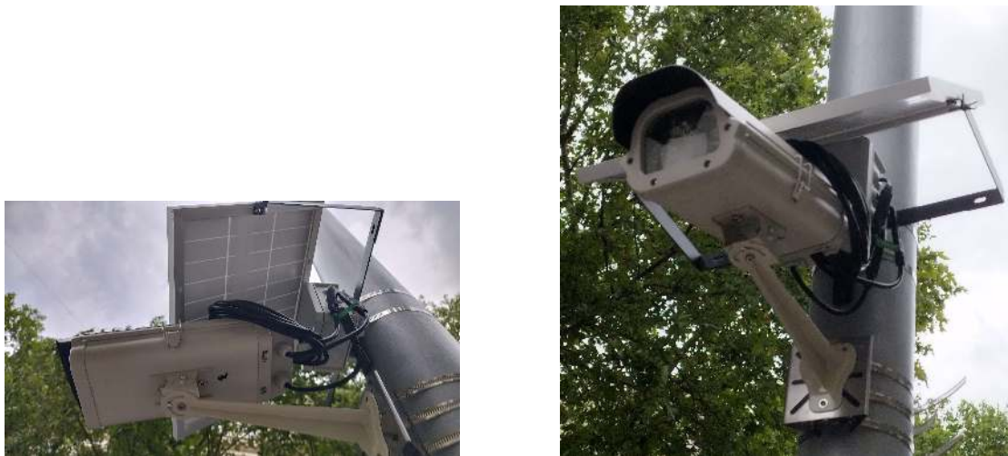
Figure 3.3: One of the two prototypes mounted on a street light pole
