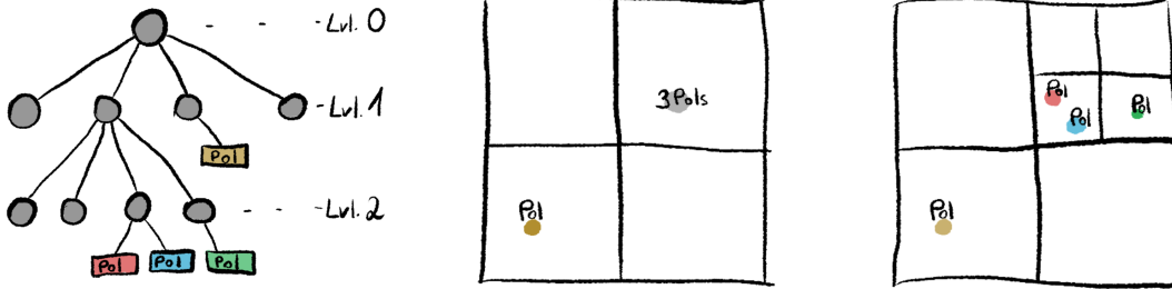
(a) Quadtree tree structure depicting three levels. (b) Top-down view at level 1; (c) One level deeper at level 2, PoIs grouped in parent nodes. with individual leaf nodes.
