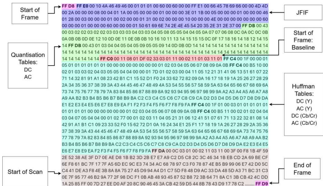
Figure 3.8: Example of a baseline JPEG file conforming to the JFIF standard. Key segments such as the Start of Image (FFD8), JFIF header, Quantization Tables (FFDB), Start of Frame (FFC0), Huffman Tables (FFC4), Start of Scan (FFDA), and End of Image (FFD9) are annotated. All markers are shown in bold, while portions of the scan data are omitted for brevity.
