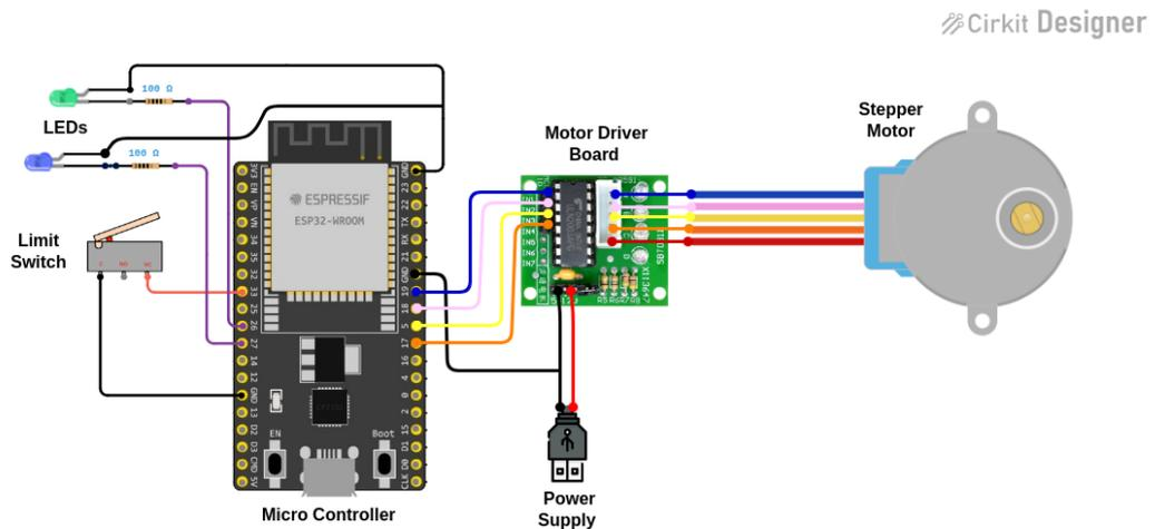
Figure 4.2: Wiring diagram: The physicalization is operated by a micro controller. LEDs and limit switch are directly connected to and powered by the micro controller, but the stepper motor is operated through a driver board and has its own power supply.
