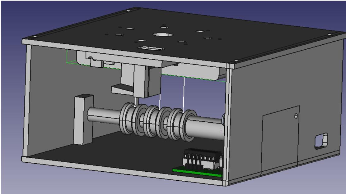
Figure 4.3: Cuboid base design consisting of a side-less bottom, a spool for the strings regulating physicalization height, a string guide and a fixture for the limit switch.
