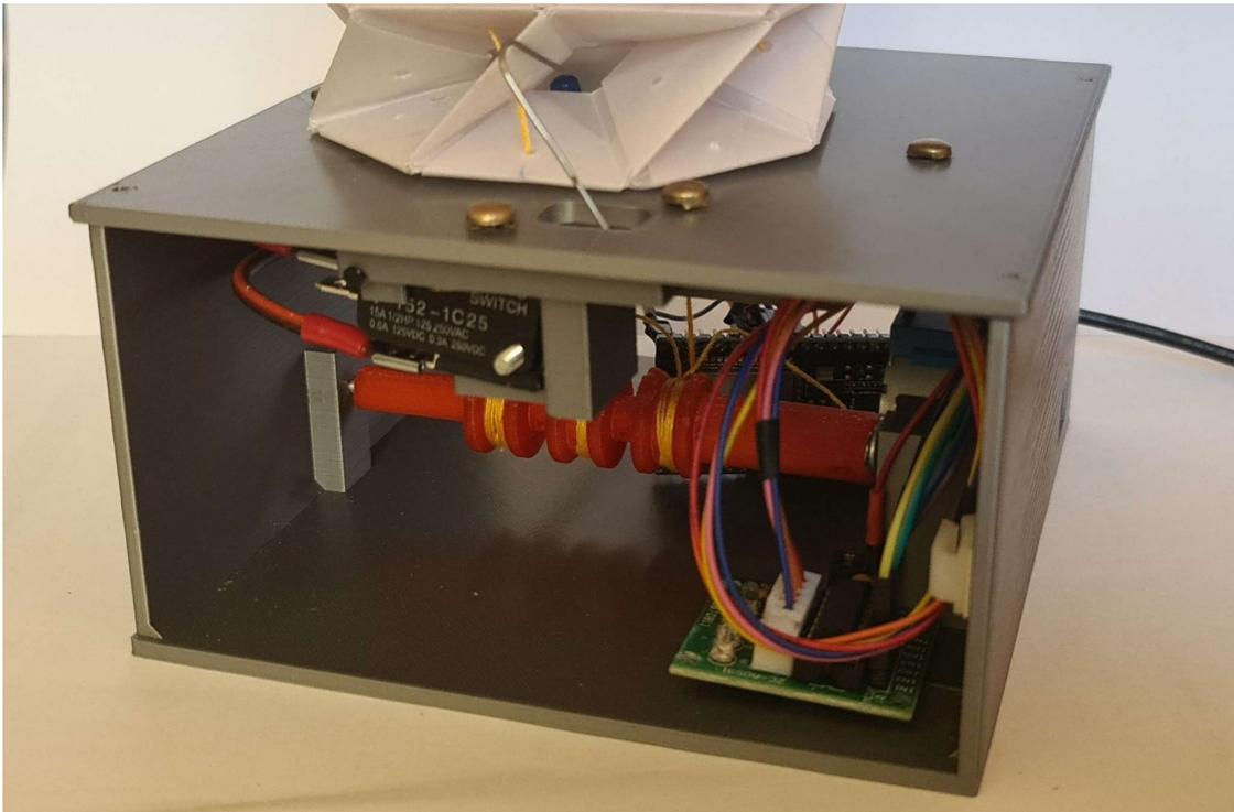
Figure 4.4: 3D-printed cuboid base containing electronics, connecting wires and paper tower on top with string traded trough holes in the paper and ready for operation
