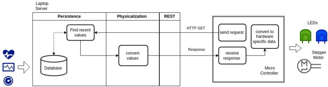
Figure 3.1: Flow diagram depicting the communication and data flow between the physicalization device and external server storing observed data.
