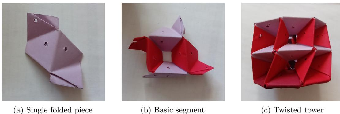
Figure 4.1: Assembly of the Origami Twisted Tower structure (c): Singular paper pieces are folded (a) and then assembled into basic segments which are then connected to each other. Eight segments in a circle make up each individual layer of the tower(c).
