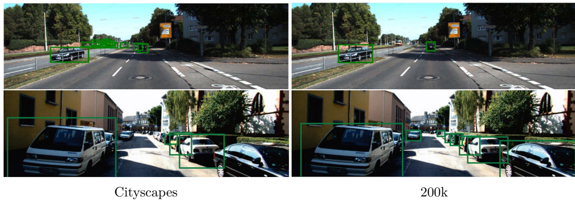
Figure 2.3: A visualization of representative detections from training on Cityscapes [COR + 16] and the dataset of 20 000 simulated by Johnson-Roberson et al. [JRBM + 16]. The simulated dataset produces less cluttered outputs and higher quality in bounding boxes.
