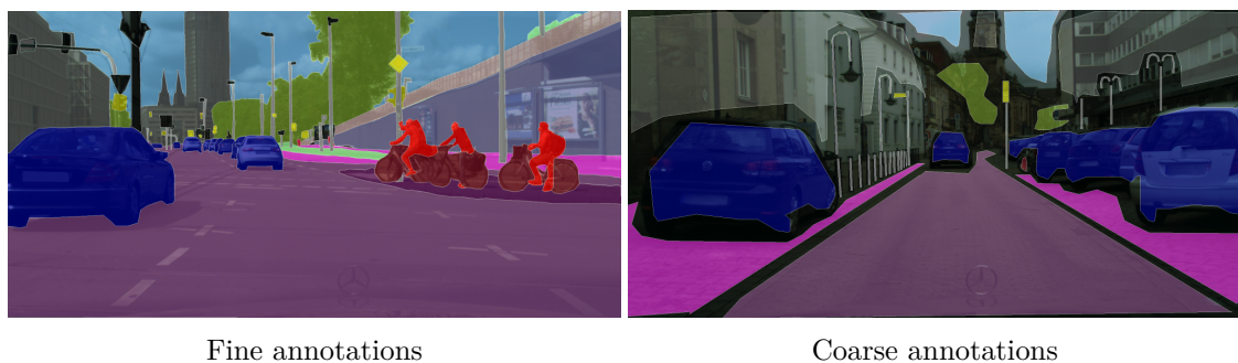
Figure 2.2: The difference between the fine and coarse annotations of the Cityscapes dataset [COR + 16].
