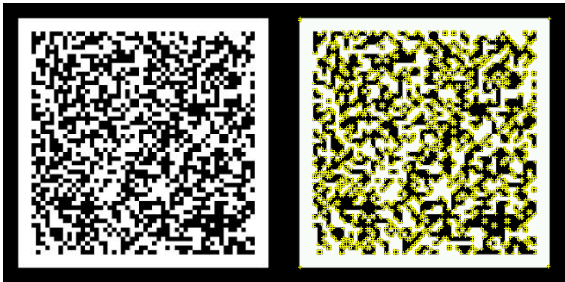
Figure 2.2: A randomly generated QR-code (left), where features are displayed as yellow crosses (right). It is easy to see, why vertices are best used for feature detection.
