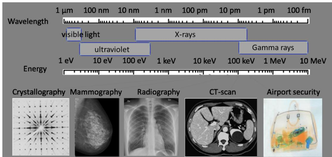
Figure 3.1: Part of the electromagnetic spectrum with wavelength and energy of visible light, ultraviolet light, X-rays and gamma rays. Taken from [Shr18].
