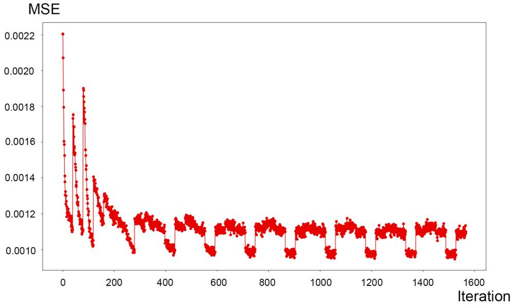
Figure 5.5: Plot of the MSE (loss function) development during our reconstruction. The x-axis is showing each optimization iteration step. As we are optimizing in 40 iterations during one  $45^\circ$ -rotation, and terminate the software after 40  $45^\circ$ -rotations, there are 1600 iterations in total. The spikes during the first full  $360^\circ$ -rotations are a result of wrong geometric assumptions of our optimizer due to not having seen the specimen from each angle yet.
