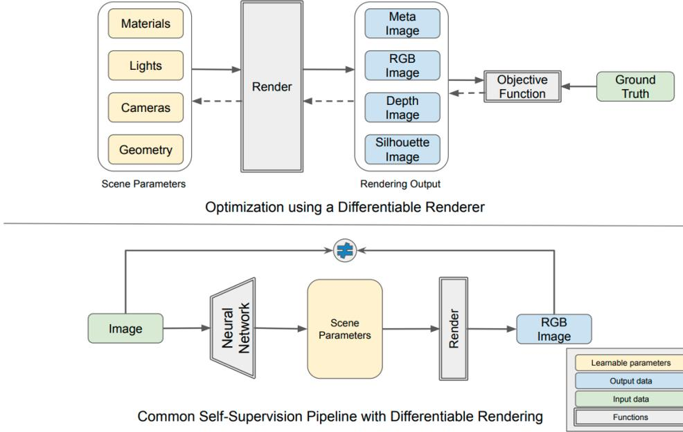
Figure 3.5: Differentiable Rendering pipelines. Taken from [KBM<sup>+</sup>20].
