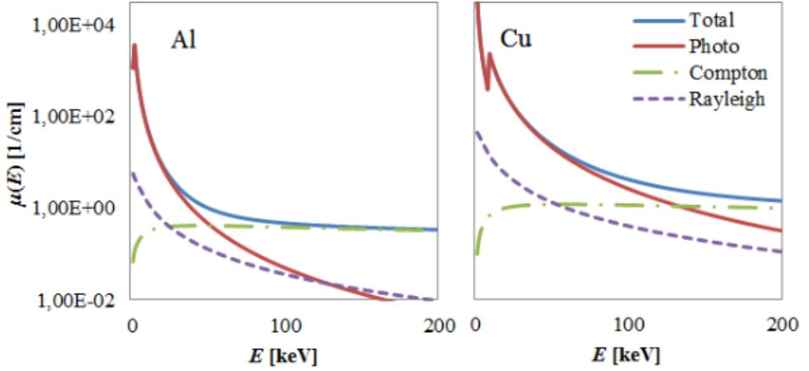
Figure 3.2: Linear attenuation coefficients of aluminium ( $Z = 13, \rho = 2.694g/cm^3$ ) and copper ( $Z = 29, \rho = 8.94g/cm^3$ ).  $Z$  denotes the atomic number of the element, and  $\rho$  denotes its respective density. Taken from [RHS<sup>+</sup>10].
