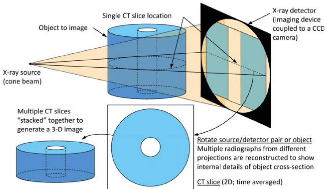
Figure 2.1: A schematic representation of a CT scan, displaying the three components (X-ray source, specimen, detector) and their role in CT imaging. Taken from [Hei11].
