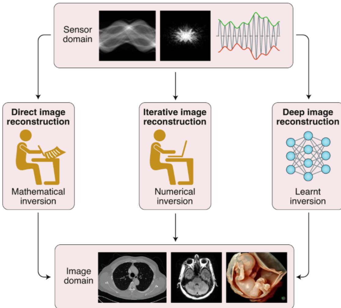
Figure 2.3: Different approaches to reconstruction for CT imaging. Taken from [WYDM20]
