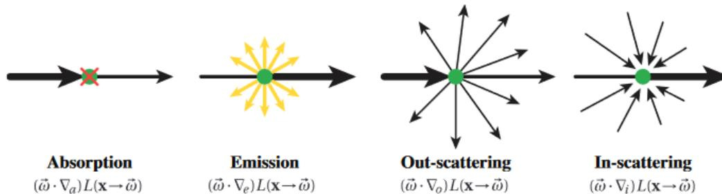
Figure 3.4: An illustration and the underlying equations for the different types of interactions a photon can have with the medium. Taken from [Jar08].
