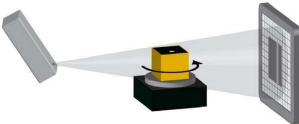
Figure 4.1: Usual CT-simulation scene setup. The X-rays are emitted through the use of a cone beam, the object is being rotated on a table and the detector is capturing the resulting energy on its flat surface. Taken from [RHS<sup>+</sup>10].
