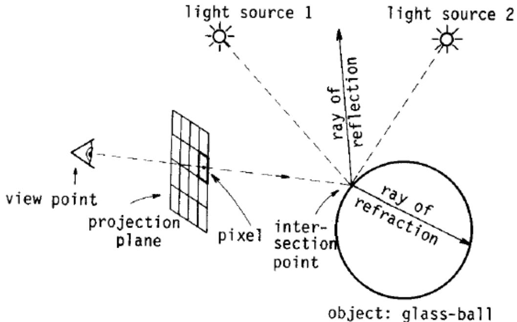
Figure 3.3: A schematic representation of a Ray Tracing Algorithm. For each pixel in the output image, a ray is being shot into the scene, which either intersects with an object or does not. The color of the pixel then depends on the intersecting object’s material, the light illuminating it, and rays of reflection/refraction reaching the intersection. Taken from [SML88].
