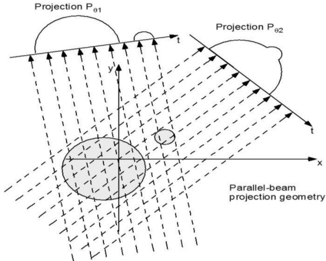
Figure 2.2: Filtered Backprojection: Acquisition of projection data from different angles. Taken from [KH16].
