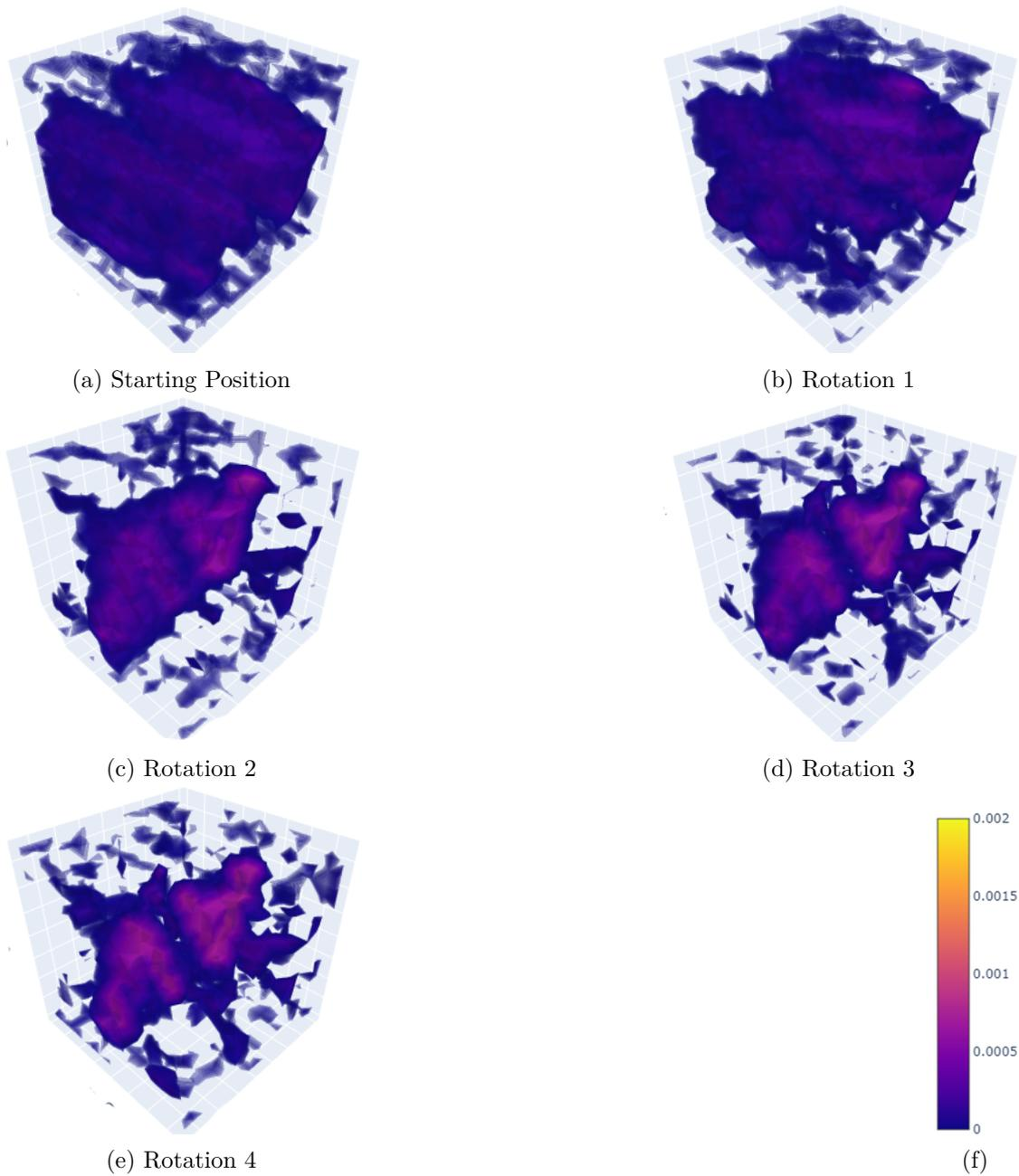
Figure 5.1: A simple volume rendering visualization of the optimized absorption coefficient matrix. a represents the volume grid after the first optimization iteration and effectively shows how optimizing the volume data from a single view/angle is not sufficient for a correct approximation. The colors of the voxels correspond to the absorption coefficient that was optimized at that voxel, as seen in f
