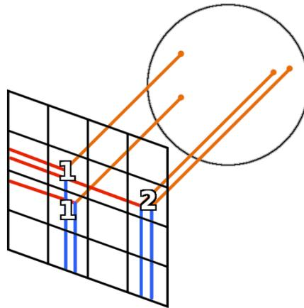
**Figure 1.3:** Projecting photons into a 2D grid. After projecting into screen-space (screen width and height of projection in the figure are set to 4, same as grid size), a point's x- and y-coordinates are rounded to the nearest integer to find the cell position.
