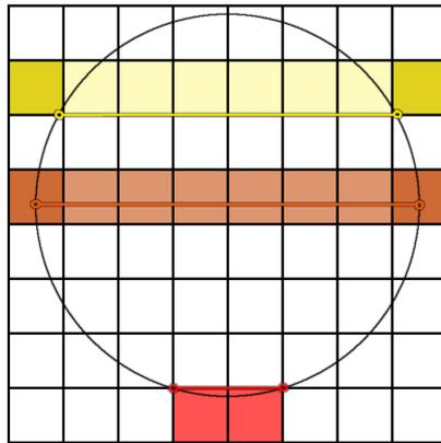
**Figure 4.1:** Width calculation; yellow: since we need the lower border we need to add 1 to get the y position with the largest width; orange: at the center we use the full radius
