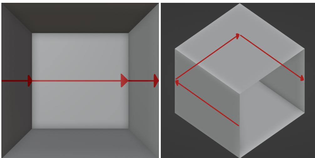
(a) For the 3D grid 94 cells are traversed (32 positive z, 31 positive x then 31 negative z) (b) In the projected space a large amount of cells are traversed (ca. 250), making cached photons become obsolete more quickly
