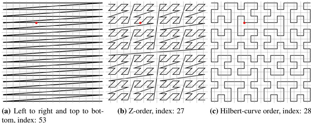
**Figure 3.1:** Different hashing function output for coordinates (5,3)
