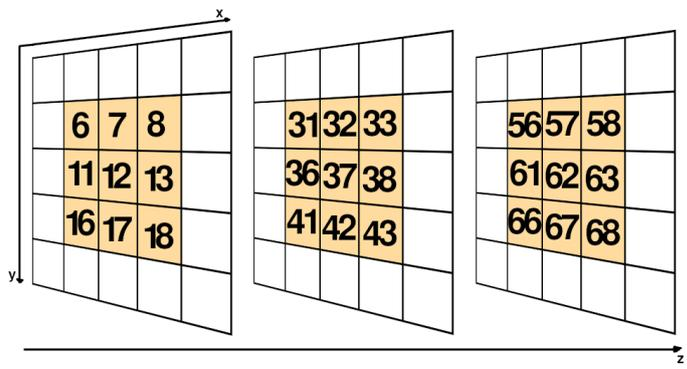
**Figure 1.2:** Spatial locality of the 3D grid. Searching through a 3 by 3 by 3 area sequentially, the memory location jumps 3 times as much compared to in a similar 2D grid.
