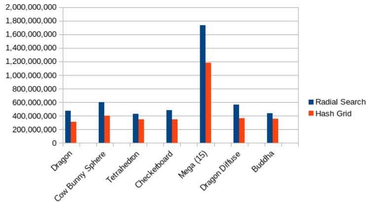
**Figure 6.11:** Read accesses per frame to the photon data structure during search
