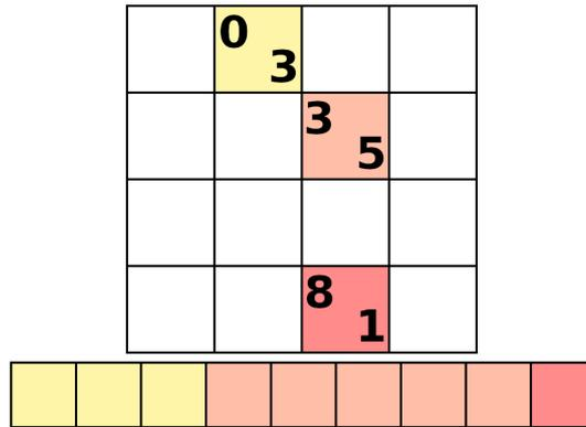
**Figure 1.1:** Example of a packed array, here a 2D coordinate is used to find a cell which then contains an index (upper left) and length (lower right) to describe an area in the packed array, empty cells would contain a length of 0
