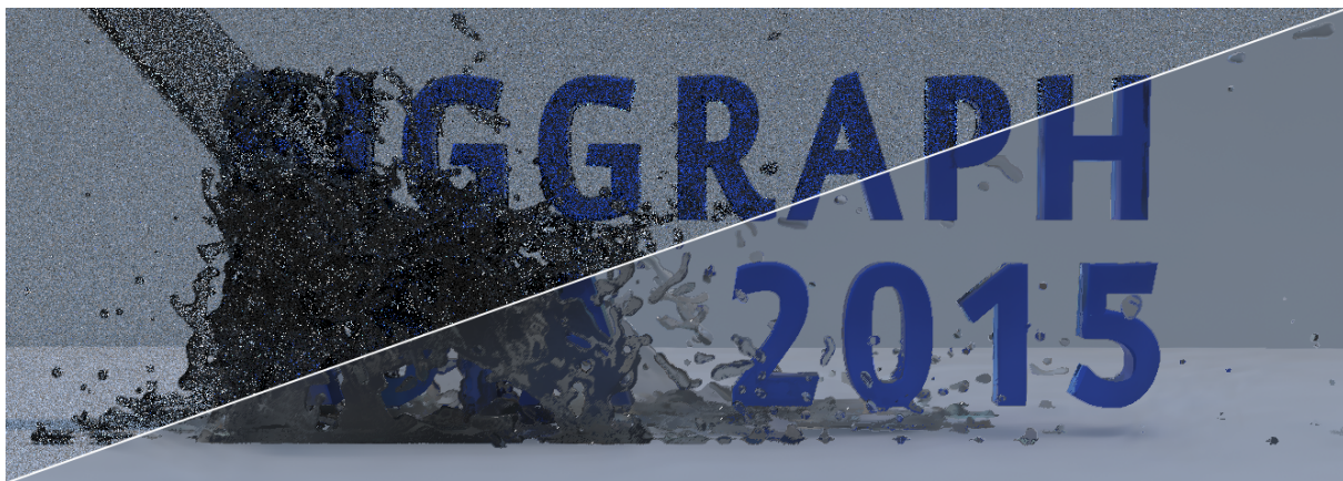
Figure 1: Our noise filtering framework is capable of rapidly denoising images rendered with a low number of samples (2 spp in this example), even in the presence of high-resolution geometry and multiple refractive materials. Our techniques are compatible with all common high-dimensional filters.
