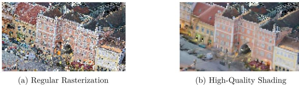
Figure 5.2: Two compute shader approaches: One displaying the closest point, the other blending overlapping points together.
