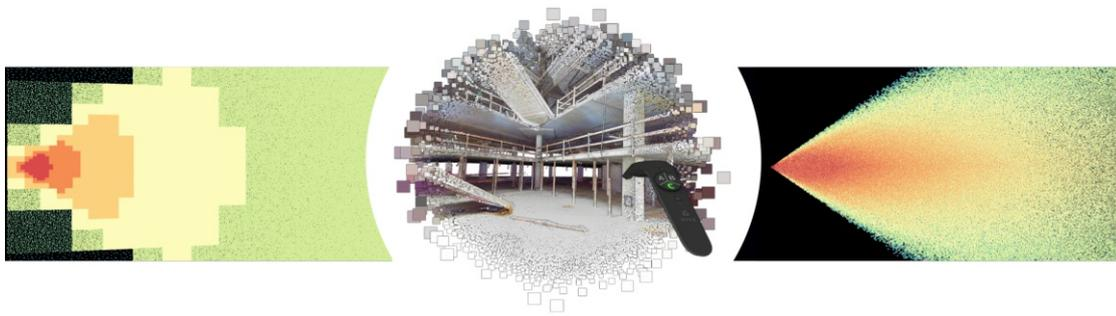
Figure 4.1: Continuous level of detail attempts to achieve gradual transitions from high levels of detail to lower levels of detail depending on distance to the viewer and distance to the center of the screen. Our targeted use case are VR applications where classic discrete LOD structures are especially noticeable due to sudden drops in point density and popping artifacts during motion.
