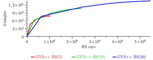
(d) Zoom-in of the first five seconds of GVS++ on the PPLANT scene using three different RS parameter configurations (GVS++ RS( $n_{RS\text{Edge}} = n_{RS\text{Area}}$ )). The number of triangles found per RS ray largely overlap. With RS(20), GVS++ found 6.4% more triangles than with RS(5) within the same time frame.
