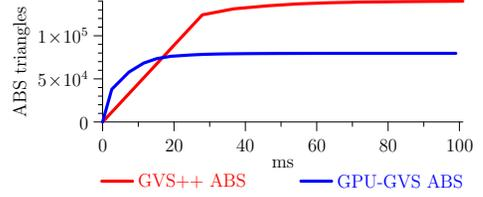
(b) The number of intersected triangles plotted over the measured ABS execution time.
