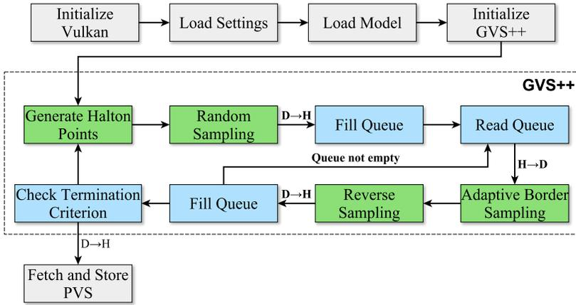
Fig. 5. An overview of the implementation of GVS++. Green boxes represent components that are implemented on the device. Blue boxes are components that are implemented on the host side. The Halton point generation, as well as random sampling, are implemented as separate shaders. The adaptive border and reverse sampling are realized as a single common shader. D→H and H→D show that data is transferred from device to host and vice versa.
