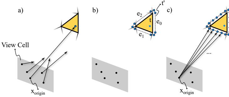
Fig. 2. The adaptive border sampling procedure is shown. Random sampling is used to find initial triangles (seed points) (a). Adaptive border sampling enlarges the boundary of the current triangle  $t$  to get a 9-vertices polygon  $t'$  (b). Additional samples are placed along the edges  $e_0, e_1$  and  $e_2$  of  $t'$ . Starting from  $x_{origin}$ , rays are traced to the nine vertices that form  $t'$  and to the samples along the edges  $e_i$  (c).
