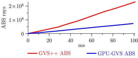
(a) The number of traced ABS rays are plotted over the measured ABS execution time.
