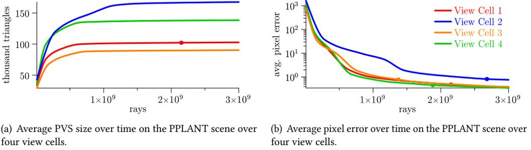
Fig. 9. PVS size (a), and average pixel error (b) over the number of traced rays for four view cells of PPLANT. Each line represents a view cell. A dot represents the used termination criterion of 10.
