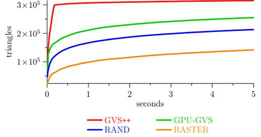
(b) Zoom-in of the PVS size over time for the first five seconds of each algorithm on the PPLANT scene.
