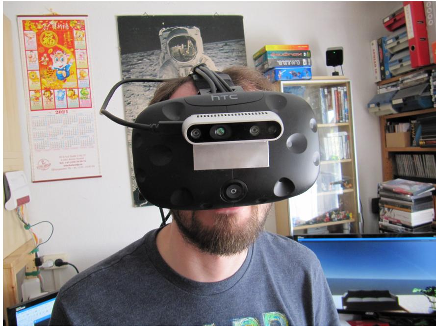
Figure 5.5: **User Study Setup:** The VR headset had the Intel Realsense mounted on it, placed on the front where it could not occlude the headset’s sensors.
