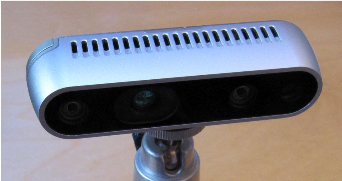
Figure 4.4: Intel Realsense Depth Camera D435
