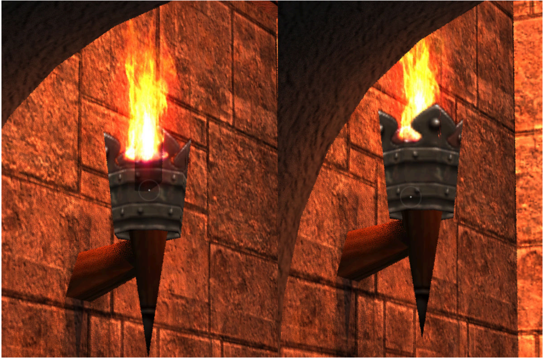
Figure 6.1: The left image shows a scenario where the transparent surface (flame) behind the metal parts leaks through since the order of the objects for which the any hit shader gets executed is random, and therefore objects behind a opaque surface can also be included. The right images shows the scenario where the maximum ray length is the exact length from the camera to the metal ring and therefore only objects between the camera and the metal ring are considered for the transparency calculation.
