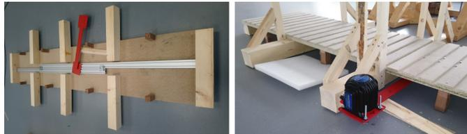
Figure 4.2: Left: Audio transducer mount on the flat bridge prop: Underside of the walkway with aluminum rail; Right: audio transducer mounted on metal arm.
