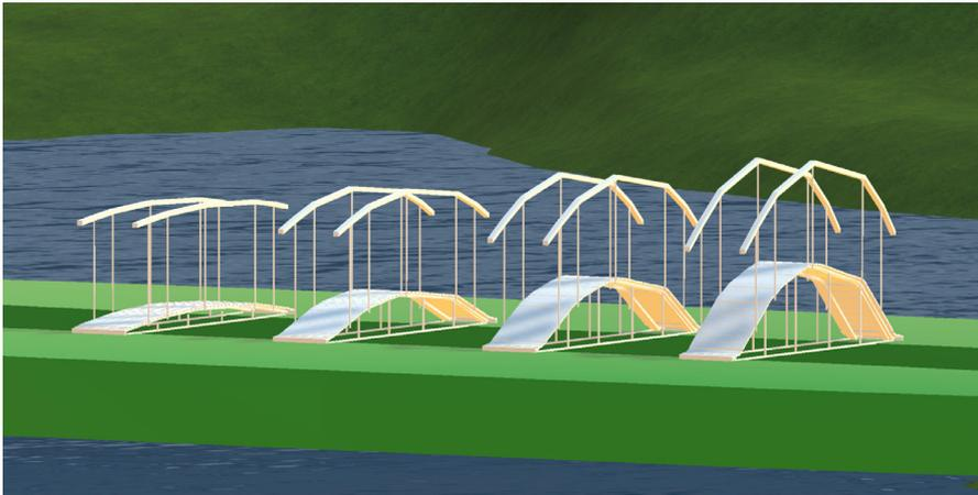
Figure 6.7: Showcase of the different visual heights of the virtual bridges used in study 2. From left to right: 10 cm (with -20cm height adjustment), 30 cm (ground truth, identical to physical bridge prop, without height adjustment), 50 cm (with +20 cm height adjustment), 70 cm (with +40cm height adjustment).
