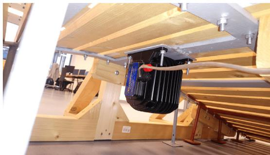
Figure 4.5: Supporting welded steel arch structure and audio transducer mount on the underside of the curved bridge prop.
