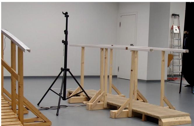
Figure 4.16: Tripod with Vive tracker used to fix floor height in SteamVR.
