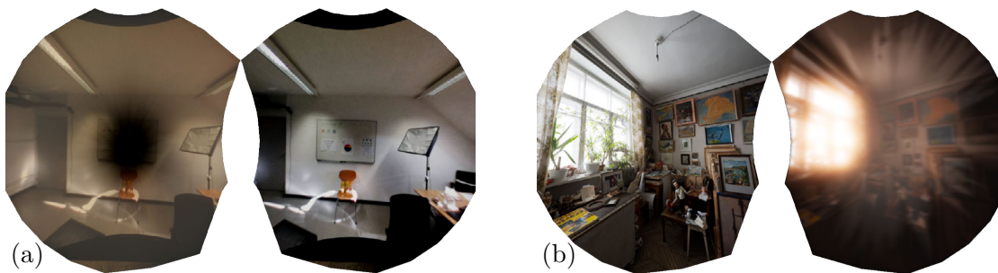
Figure 9.1: Simulation of cataract vision in eye-tracked stereoscopic head-worn display. Study participants were cataract patients with one corrected eye and one uncorrected eye. (a) Posterior subcapsular cataract simulated for corrected left eye and no modification for uncorrected right eye, viewing live stereoscopic video. (b) Cortical cataract with glare simulated for corrected right eye and no modification for uncorrected left eye, viewing 360° image.
