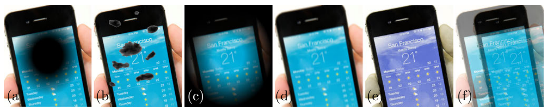
Figure 4.6: AR simulation of (a) macular degeneration, (b) diabetic rethinopathy, (c) glaucoma, (d) cataracts, (e) protanopia (color blindness) and (f) diplopia (double vision) by Ates et al. For these visualizations the authors applied their developed filters onto 2D images, using a VR media player. We can expect a significantly blurrier image when viewed on the Oculus Rift, due to the resolution of this HWD, also mentioned as limitation by the Ates et al. Reprinted from [AFF15].
