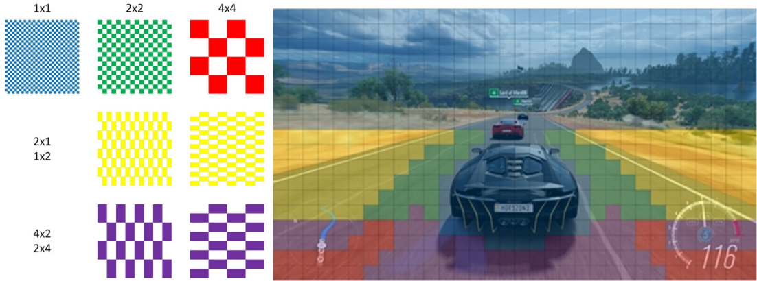
Figure 3.1: Supported coarse shading rates with an example of VRS in a racing scene. Reprinted from the NVIDIA Turing architecture whitepaper [NVI18].
