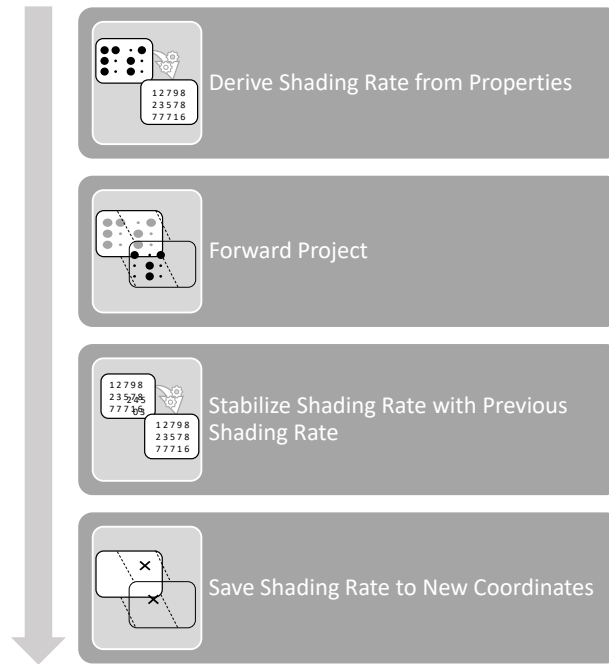
Figure 4.2: The common steps for the computation of the shading-rate image. First, the shading rate is derived from the properties. This process depends on the used properties. In the next step, the coordinates in the next frame are computed by a forward projection. Finally, the shading rate is stabilized by our TAA-based approach and saved to the new coordinates.
