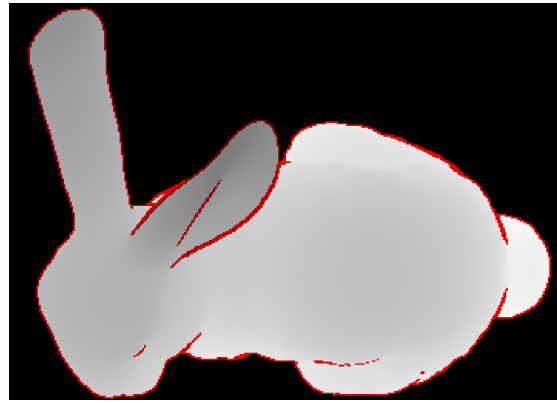
Figure 3.5: Range scan image with occlusion pixels marked in red.
