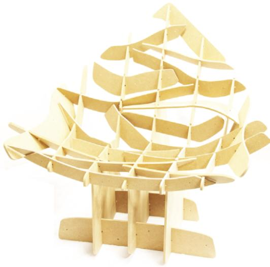
Figure 2.3: Chair built from interlocking parts created by the system from Schwartzburg and Pauly [SP13].
