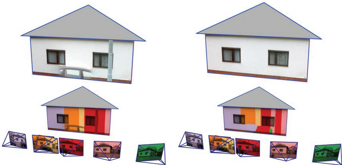
Figure 6.7: Top left: The initial texture containing occluders. Bottom Left: The associated shots, visualized using a false color mask. Top right: The cleaned texture after interactive brushing. Bottom right: The correspondingly modified mask.
