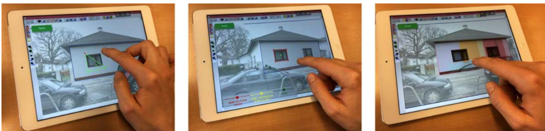
Figure 6.8: Evaluation of our proposed system on a touch-based device. Left: Coarse sketching of the polygon in the initial view. Middle: The polygon has been snapped to image edges and been reprojected to a neighboring image in the multi view sketching mode. The visual guidance feedback indicates that enough views have been used. Right: Interactive brushing.
