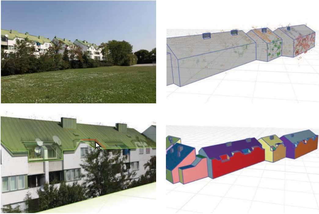
Figure 5.12: Reconstruction of a building complex occluded by trees and bushes. Top left: An example photo of the data set. Top right: The segments extracted from the sparse point cloud (obtained from a photogrammetric approach) and the main structures after approximately three minutes of optimization-aided modeling. Bottom left: The reprojected images help the user to modify the polygon boundaries and to sketch new polygons forming the balconies. Bottom right: The final model after 20 minutes using the additional image information.
