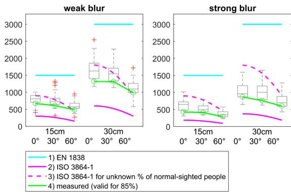
Figure 3: Comparison of our measurements of recognition distances to different norms and standards. Reprinted from [4]
