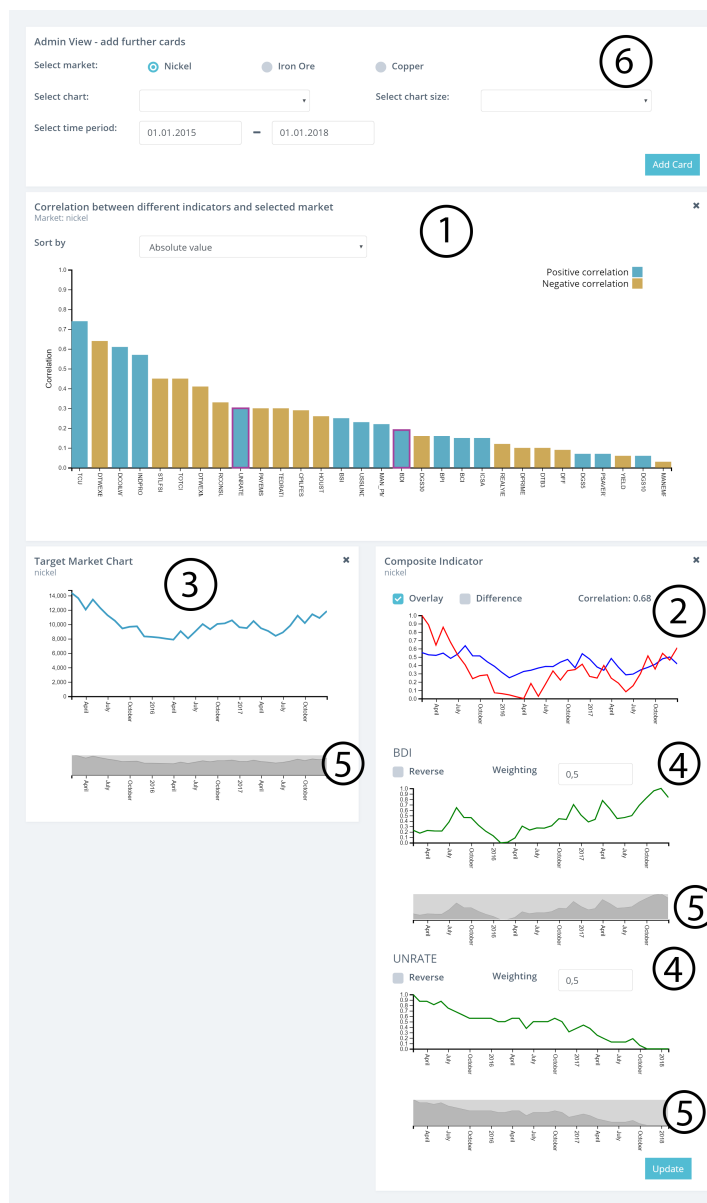
Figure 4.3: Default dashboard configuration including (1) CC ranking, (2) CI, (3) target commodity market chart, (4) indicator charts, (5) navigation charts and (6) Admin View.
