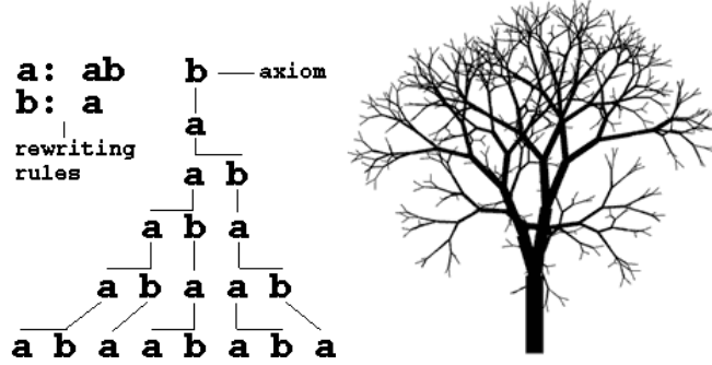
Figure 3.2: Left: an example of L-Systems rules and derivation. Given two rules and an axiom shape, derivation allows generation of infinite number of sentences in this manner. Right: a tree generated with an L-System (courtesy of Ted Wong, Bryn Mawr College).
