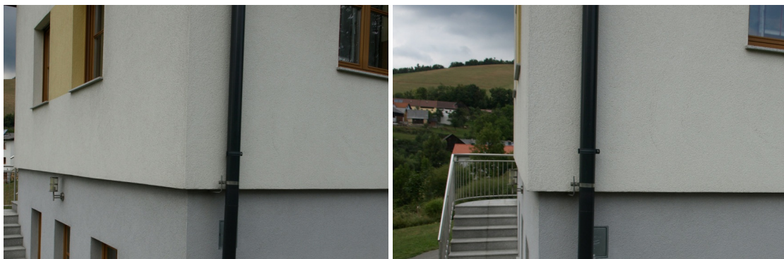
Figure 4.3: A small baseline is necessary around house corners because a mere small change in viewpoint makes for a large change in perspective.
