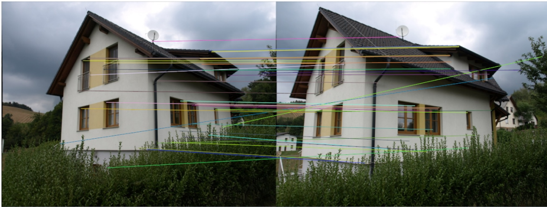
Figure 4.4: Brute force matcher. Matches are few in number, and mismatches often come from vegetation in the image. Matches are visualised as coloured lines.
