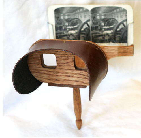
(b) A stereoscope projects two photographs from slightly different viewpoints into the left and right eye. This creates a sense of three dimensional form. Source: [Hol]
