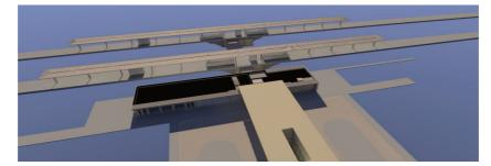
Fig. 2: Daylight simulation for a train station. Both direct sunlight as well as ambient light are simulated, and multiple light bounces are considered. The light transport computation in this scene took approximately 20 seconds
