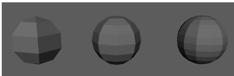
Figure 3.1: Spheres with different level of detail. From left: 40 triangles, 112 triangles, 264 triangles
