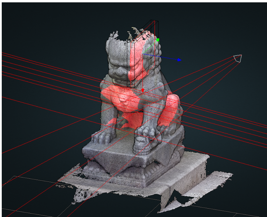
Figure 3: The lion point cloud is clipped by a clipping plane, a perspective clipping polygon and an orthogonal polygon.
