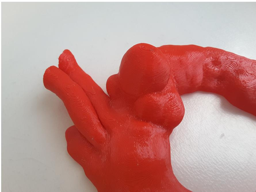
Figure 6.2: Close-up of 3D print from a segmented aorta. The uneven surface leads to a better perceived quality, even though printer and printing parameters were the same as for the fixed-diameter print (compare with Figure 5.1 and 5.2).
