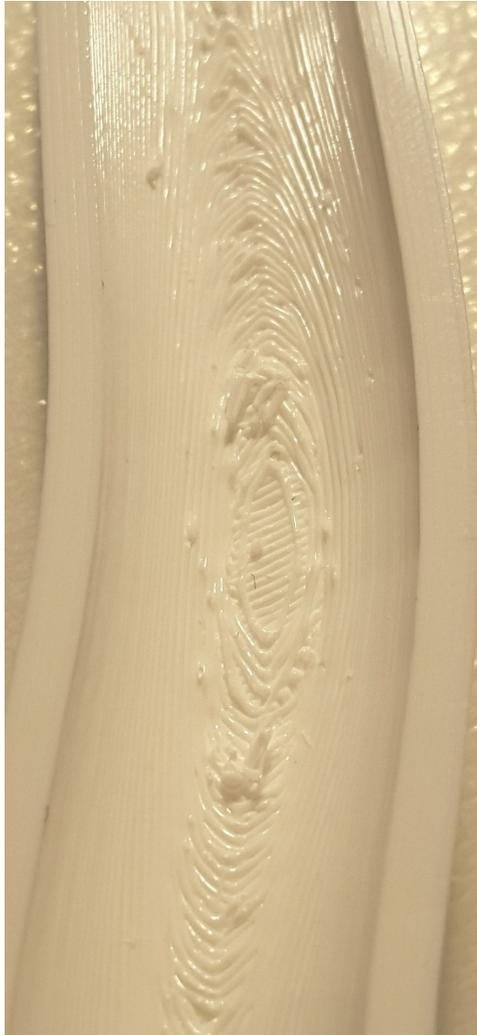
(a) Surface of the tube's inner shell. While the surface is very smooth at the sides of the tube, it gets rougher towards the middle where support material was needed.
