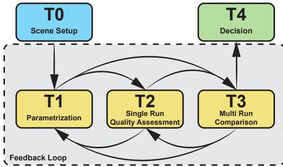
Fig. 3. The five steps of the lighting designer's workflow. After initialization of the scene (T0), the lighting designer works in an iterative fashion (T1-T3) until he or she finds a satisfactory solution (T4).
