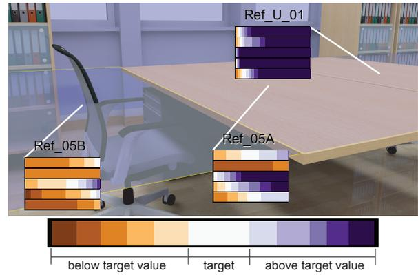
Fig. 5. Measurement Surface Annotations displaying illumination distribution histograms for five selected simulation runs. The annotations enable the comparison of abstracted illumination values in a spatial context across multiple measurement surfaces and parametrizations.
