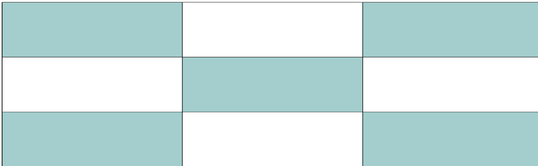
Figure 3.7: Example of how the rectangles are placed in the area control term. The blue tinted rectangles are the ones enlarged until the appropriate amount of nodes is placed inside them. Note that the height and width of the input bounding box are divided by 3 to get the correct placement of the lines forming the rectangles.
