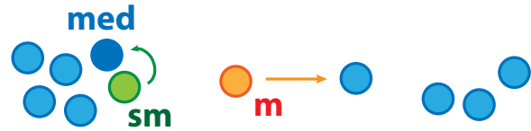
Figure 6: Ensemble medoid. The input volumes can be interpreted as points in a k -dimensional space (in blue). The mean ( m ) is usually prone to follow outliers in the dataset, and the nearest neighbor (arrow) of the mean would not be a good representative of the dataset in this case. The spatial median ( sm ) minimizes the Euclidean distances to all points, but is generally not a part of the dataset. We therefore find the point that is closest to the spatial median (arrow) and use this as the medoid ( med ) of the ensemble.
