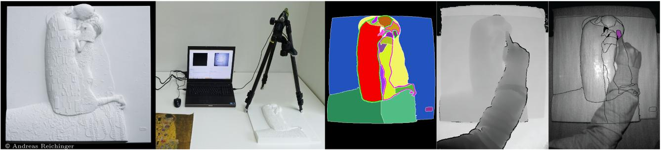
**Figure 1: From left to right: a) Tactile relief interpretation of Gustav Klimt’s “Der Kuss” (The Kiss, 1908/09); b) Test setup; c) Label image, warped to camera space. Outlines indicate merged base labels; d) Depth image; e) Infrared image with superimposed label borders and touched label (purple). © Andreas Reichinger**
