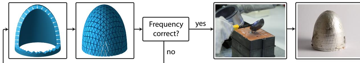
**Figure 1:** The optimization loop works on offset surfaces and evaluates the incumbent solution using a finite element mesh. Once the optimal wall thickness for a given pitch is found, we cast the result using sand molds and tin.
