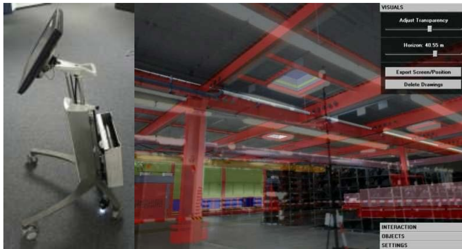
Figure 2 (left) The Planar is a touchscreen display on wheels, which can be used (right) for discrepancy analysis directly in a factory hall.
