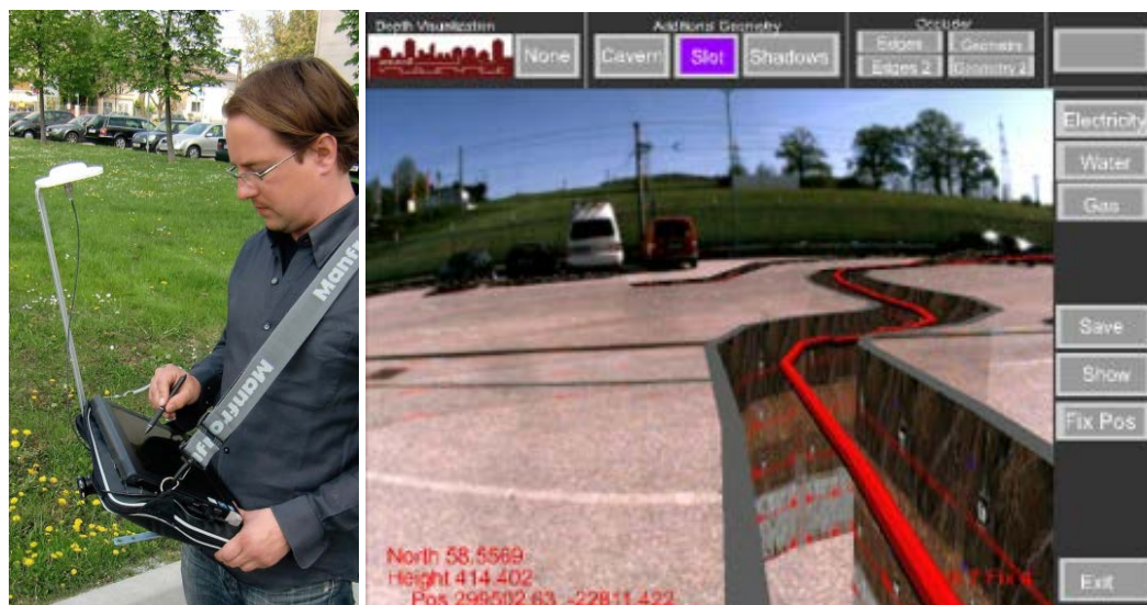
Figure 3 (left) Tablet computer with differential GPS system for outdoor AR. (right) Geo-registered view of a virtual excavation revealing a gas pipe.
