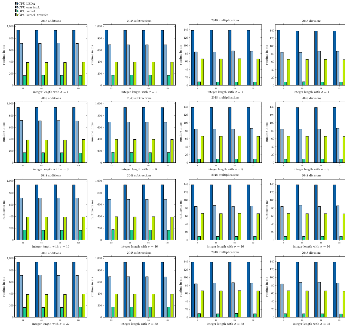
Figure C.7: Benchmark timings for 2048 rational number computations addition, subtraction, multiplication and division. On the x-axis are the lengths of the nominator and denominator in multiples of 32 bit. The deviation of the length of the nominator and denominator are in each row from \sigma = 1 to \sigma = 32 .
