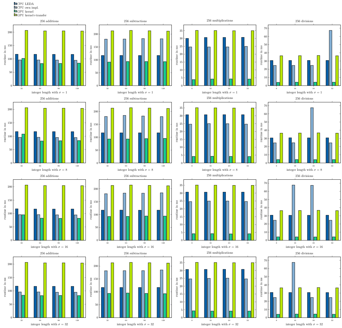
Figure C.4: Benchmark timings for 256 rational number computations addition, subtraction, multiplication and division. On the x-axis are the lengths of the nominator and denominator in multiples of 32 bit. The deviation of the length of the nominator and denominator are in each row from \sigma = 1 to sigma = 32 .
