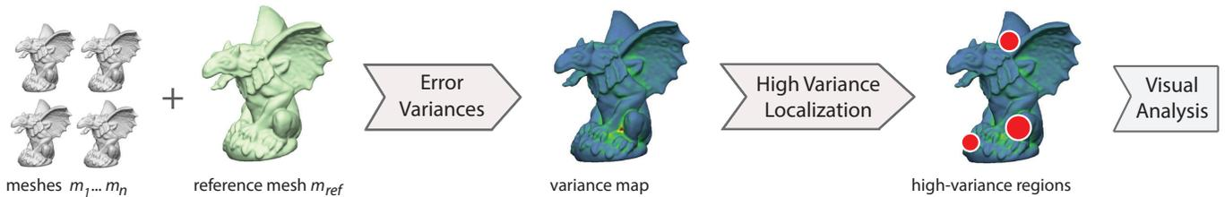
Fig. 3: Overview of our visual analysis approach. The input data consists of a set of  $n$  meshes and one reference mesh. The surface deviations of the meshes are calculated to get the corresponding variance map (Section 4.1). Afterwards high-variance regions are located in the data (Section 4.2). The results are finally presented in an interactive visualization as described in Section 4.3 and Section 4.4.
