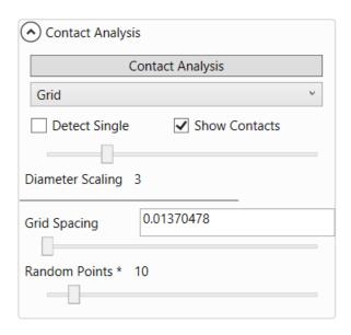
The image above shows the UI Settings for the contact detection algorithm. The combobox selects the algorithm that is used for contact detection:
