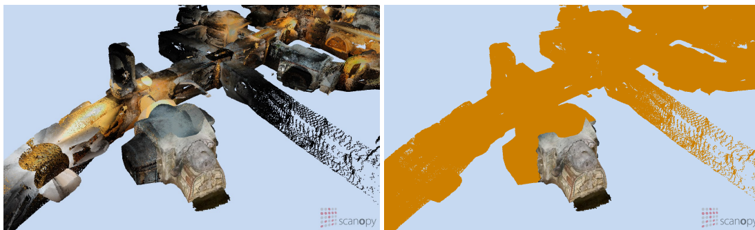
Figure 5.2: The cubiculum of the Fossor Diogenes [113] in the context of the adjacent hallways. The hallways are rendered as point cloud, while the photos of the paintings in the cubiculum are stored in a virtual texture, which is mapped onto a mesh model. In the left image, the virtually textured mesh is blended into the point cloud, while in the right image, the point cloud is marked, so the virtually textured mesh can be easily distinguished.
