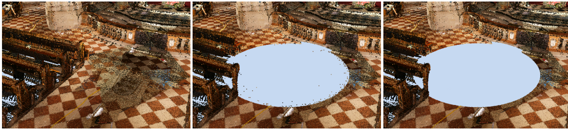
Figure 3.19: From the original point cloud (left image) a spherical volume is deleted. The center image shows the artifacts that remain when the interior nodes are not updated after deleting points. In the right image, the points in the interior nodes have been updated according to the deleted volume.
